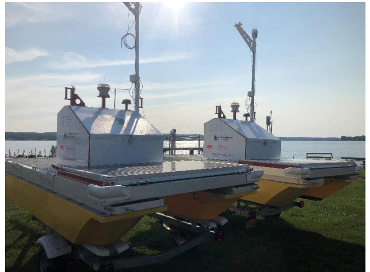
Photo 2. Two Rensselaer Polytechnic Institute-built vertical profilers prior to deployment on Chautauqua Lake. (Source: Alliance)
